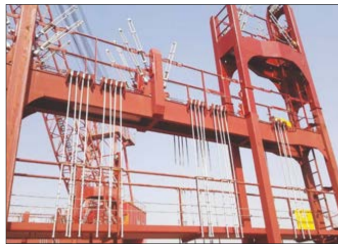
MacGregor believes that better loading capacities can be achieved, in part by converting a ship's internal lashing to an external lashing arrangement
