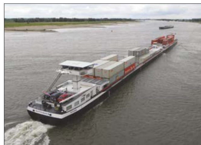
The 342 TEU dual-fuel EIGER-NORDWAND motor/push barge combination (photo: Danser Group)
