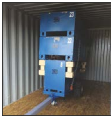
Load testing of LP's SolidStart LSL flooring
