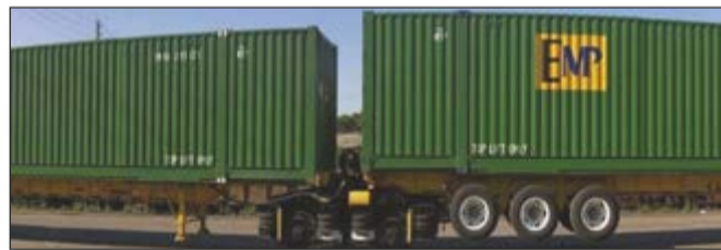
RailRunner unit in testing in the US with domestic 53ft containers/trailers
