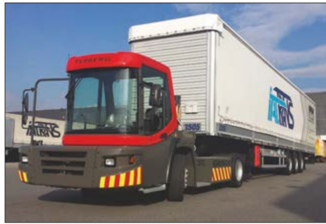
A Terberg DT223 low entry cab tractor at work in Italy
