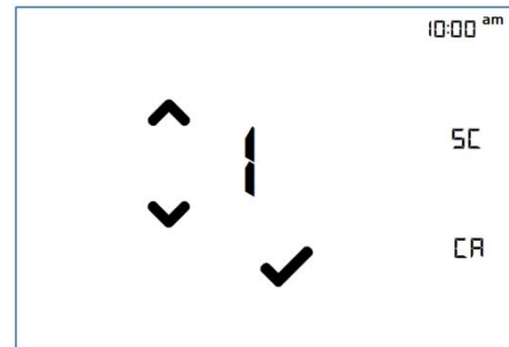
Figure 11 - Configuration Menu with Options 0-IDLE, 1-RTU, 2-HP-O, 3-HP-B
