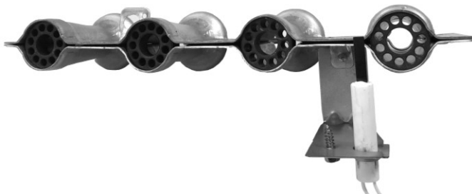
Fig. 5: Flame-side view of correct ignitor position
