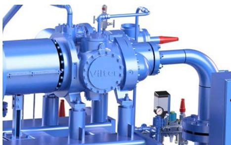
The Transcritical CO<sub>2</sub> Compressor Unit is based on proven single-screw compression technology and is equipped with on-board controls, a suction valve/strainer, an oil management system and an inverter duty motor.
